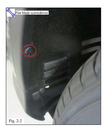
(c) Remove the fastener indicated by the circle (Fig. 2-2).
