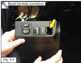
(c) Detach the harness clip and remove the panel from the vehicle (Fig. 5-3).
