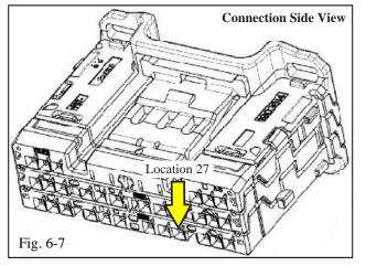
(g) Snap the lower connector shell onto the connector (Fig. 6-7).
