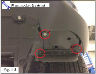
(c) Use the two (2) screws and one snap-fastener removed in Step 3(d) to install the fog light & bracket assembly in the left side and right side (Fig. 4-3).
