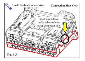
(d) Use a small flat-blade screwdriver to gently pry open the connector indicated by the arrow (Fig. 6-5).
