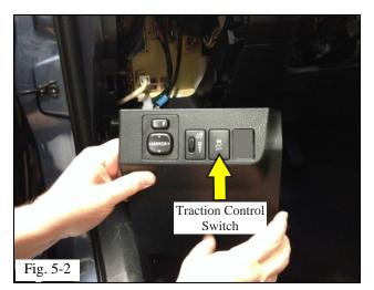
(b) Disconnect all of the connectors and take note of the traction control switch connector (Fig. 5-2).
