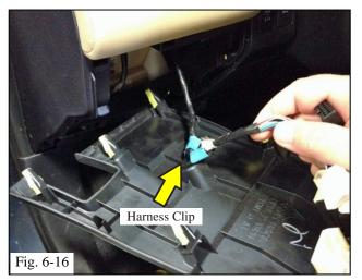
(u) Reconnect the harness clip disconnected in Step 5(c) (Fig. 6-16).
