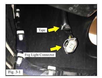
(b) Remove the tape to release the fog light harness connectors (Fig. 3-1).
